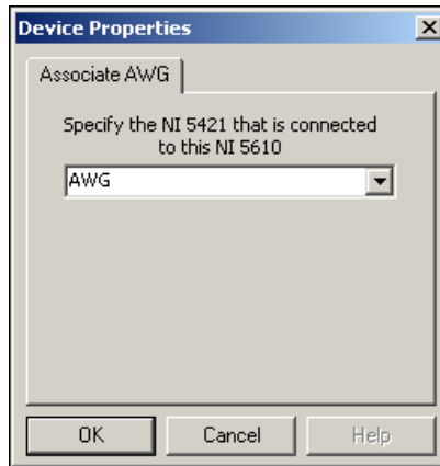
Figure B-2. The NI PXI-5610 Device Properties Dialog Displays the Associated AWG
